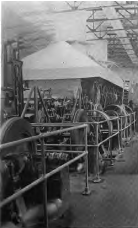
Fig. 3. Paper Machine Protection.* Protection of "back line," ventilating hood, etc., for paper machine is shown in Fig. 3.
